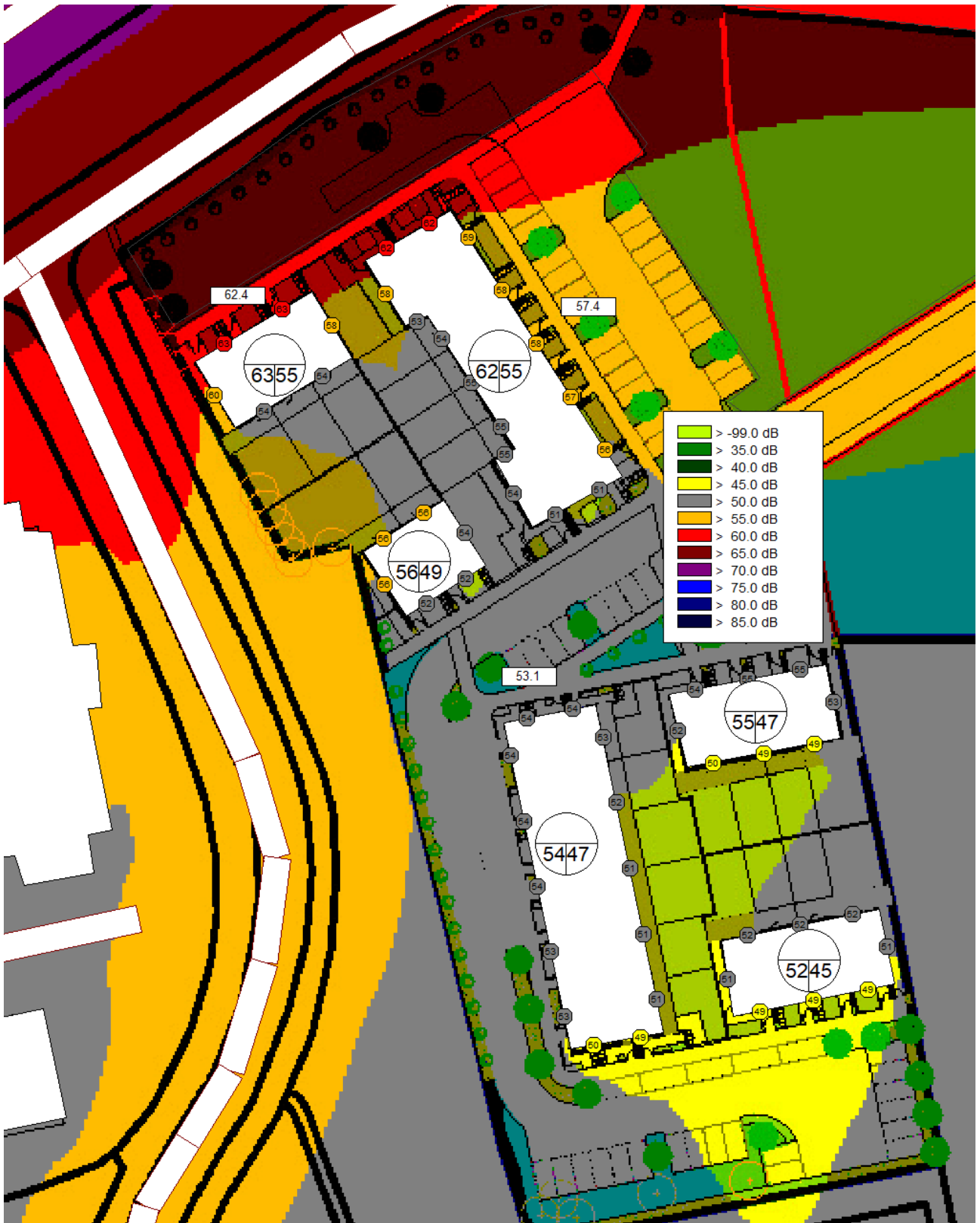
Figure 4-3 - Predicted noise levels, Lday. Receiver grid height of 4m to represent first floor level.
